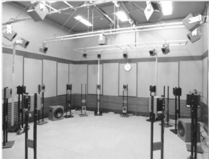
Fig. 6 Acoustic evaluation room at NHK. This room strictly adheres to Rec. ITU-R BS.1116-1.
