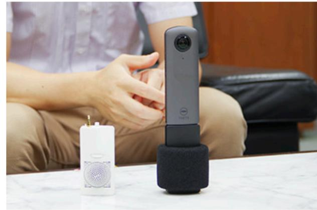
Prototype of external 3D microphone TA-1 & Wind screen attached TA-1
