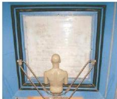
Figure 13. The Z-axis of the mannequin aligned with the center of the test panel (Test 1 in Table 11).
