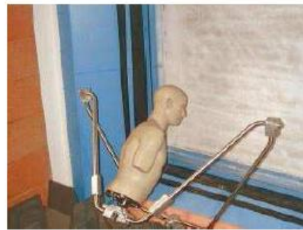
Figure 14. The KEMAR mannequin rotated 45 degrees about the Y-axis and minus 45 degrees about the X-axis (Test 8 in Table 11).
