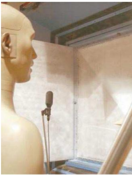
Figure 20. View of the B-format microphone at measurement location loc.1 with the mannequin in the foreground at measurement location loc.2.
