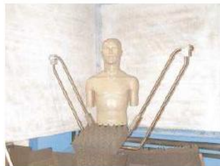
Figure 16. The mannequin rotated 150 degrees about the Y-axis (Test 4a in Table 15).
