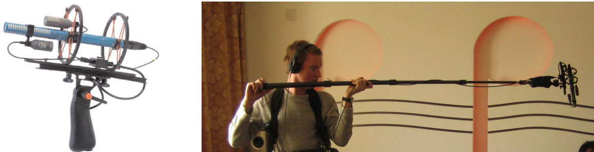
Figure 25: A Double-M/S setup with a shotgun microphone. Left: Implementation using the Schoeps Double-M/S set "CMIT" (microphones used: CMIT 5U, CCM 4 and CCM 8). Right: the setup in action ([37], photograph courtesy of André Zacher)
