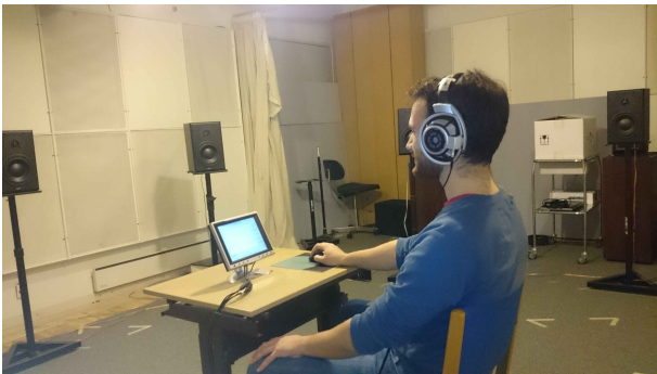
Figure 2: Photograph of the experimental setup with a listener at the listening position inside the IEC listening room. The four loudspeakers were positioned at 0, 25, 60, and 90° at a distance of 2.5 m. The listeners controlled the experiment via a graphical user interface on a small screen using a wireless mouse.
