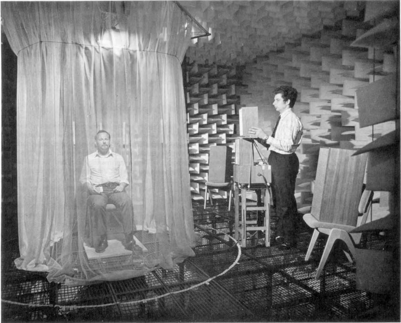
Fig. 8 - Free-field arrangement for relative sound localisation experiment
