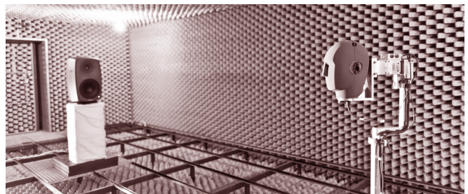
Figure 1: Genelec 8260A speaker and Neumann KU100 dummy head mounted on the VariSphear motion system [5] in the anechoic chamber. [Photo: P. Stade]
