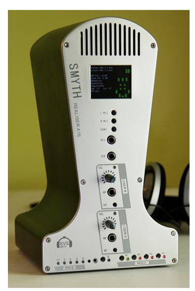
The Realiser-A16 audio processor re-creates immersive 3D audio over stereo headphones, rendering up to sixteen virtual loudspeakers in any location, with head-tracking.
