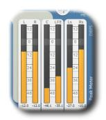
Meters for up to 6 input channels. In RMS mode peak values are displayed, in EBUR128 mode true peak values are displayed. LED signal meter range is from -60dBFS to +12dBFS, in 3dB steps. Value below meter shows maximum value. If signal clips (above 0dBFS) top LED lights red. Mouse click on one of the meters resets max, values.
