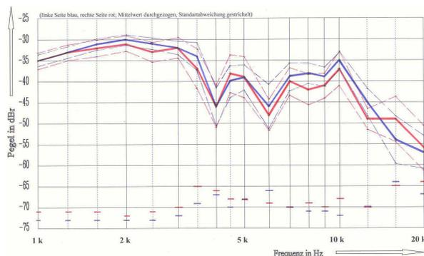
**Figure 7:** DFTF no. B1 of a supra-aural open headphone with a centric speaker, but de-centric sound source (lined); the standard deviation (dotted) and the maximum values (dashed); the left channel is colored blue and right is colored red.
