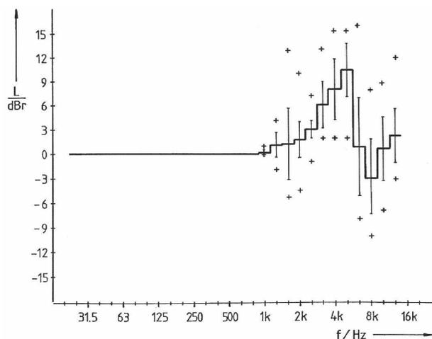
**Figure 2:** Transfer function comparison of coupler and dummy-head-measurements via 20 different headphones (lined), the third octave standard deviation "I" and there maximum variations shown by "+".
