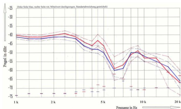
**Figure 5:** Diffus-field transfer function (DFTF) no. 4 of a circum-aural headphone with a centric speaker (lined); the standard deviation (dotted) and the maximum values (dashed); the left channel is colored blue and right is colored red.
