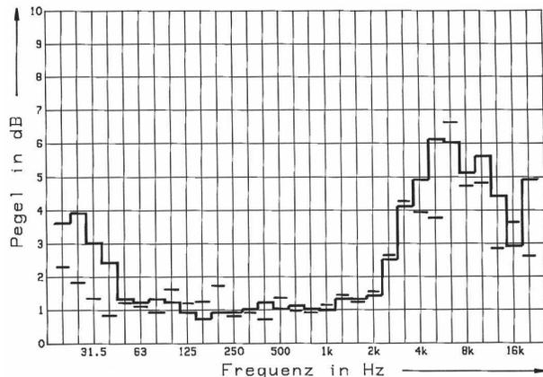
**Figure 1:** Shown outer ear third octave band variation based on two headphones measured by 8 and 16 persons each lined.
