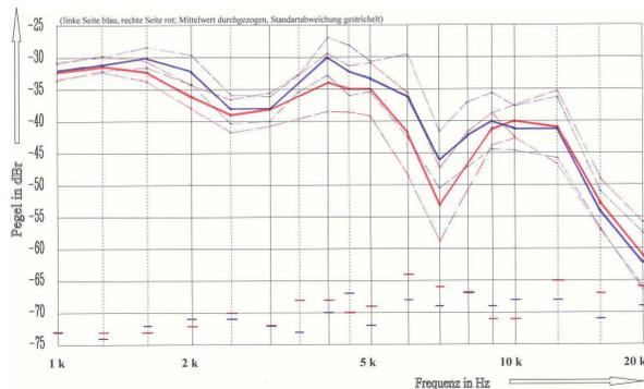
**Figure 8:** DFTF no. B2 of a circum-aural closed headphone with a centric speaker, but de-centric sound source (lined); the standard deviation (dotted) and the maximum values (dashed); the left channel is colored blue and right is colored red.
