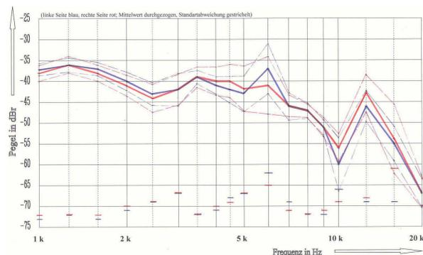
**Figure 6:** DFTF no. A3 of a circum-aural headphone with a de-centric speaker; the standard deviation (dotted) and the maximum values (dashed); the left channel is colored blue and right is colored red.
