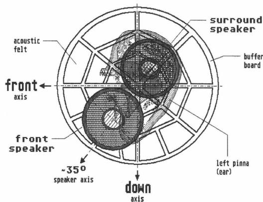
**Figure 3:** Principle of a circum-aural four channel headphone (type A) for in front localization with a main de-centric "FRONT speaker" placements based on [3]. Furthermore a de-centric speaker to reproduce REAR tone signals in the vertical hearing plain.
