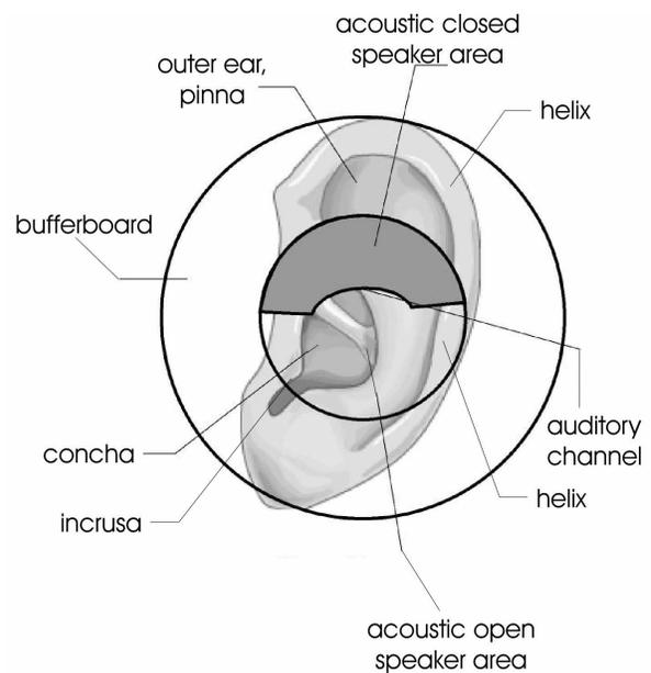
**Figure 4:** Principle of a circum-aural headphone (type B) for in-front-localization with a centric speaker placement based on [3], but a de-centric sound source at the near-field of the outer ear.
